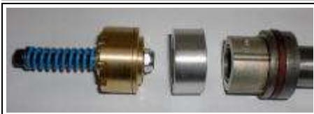
The adapter is a simple sleeve that goes between the damping rod and the Emulator. The main spring holds it all together.
