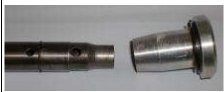
On the bottom end there is a trick bottom-out cone that has a one-way check valve. If you look carefully there is a round cross-section circlip on the damping rod just below the top (left) set of holes. This retains the bottom-out cone.
