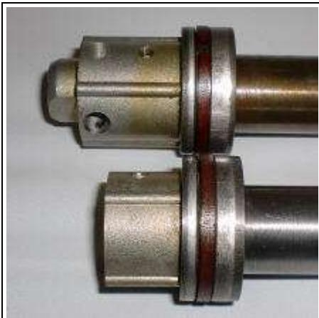
The damping rod head must be machined off flat just below the outlet holes. Remove only enough material to clean up the holes to make a flat surface. This will leave a lip of the aluminum head covering the end of the steel damping rod. This is best done on a lathe but can be done with a hack saw and a file if you are REALLY careful (don't blame me if you mess it up).
