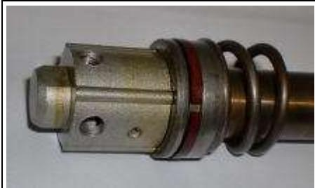
This is the stock damping rod head. The aluminum head has outlet ports exiting the sides. The head is threaded on and held in place with a roll pin. It does not have to be removed from the damping rod to modify it.
