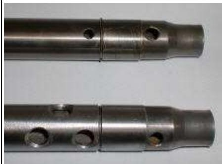
The holes below the clip (to the right) feed the one-way bottom-out cone. The compression holes are above (left) the clip groove. Enlarge the original compression holes only to 6mm (1/4"). Add two more sets of holes above (left) at 90 degrees to the last set. Carefully deburr.
